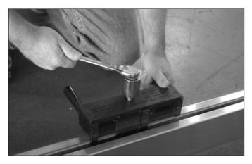
Make sure the blade movement mechanism of the TLK12 Tool moves freely, and hasn't become filled with dust or debris. Blade mechanisms that are poorly maintained may cause binding during the Taper compression operation, and result in an improper installation with insufficient compression of the Tapers.
