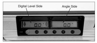
Display for Digital Level and Angle Locator.
